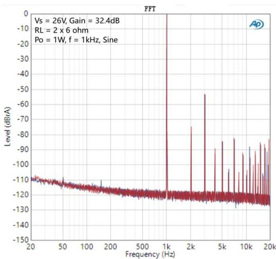
**图 15: FFT (-60 dB) (Vs = 26 V)**
