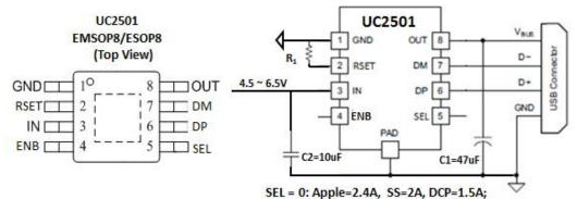
SEL = 1 or Floating: Apple=2.1A, SS=2A, DCP=1.5A; ENB is floating or pull down with 10k Resistor if not used
